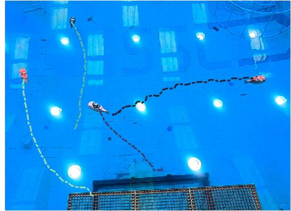
(b) Parallel formation control fish robot trajectory with IMU errors
