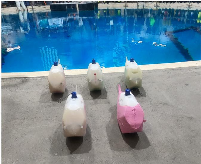
Figure 1.2: A school of soft robotic fish serves as a testbed for formation control experiments at the University of Maryland’s Neutral Buoyancy Research Facility.
