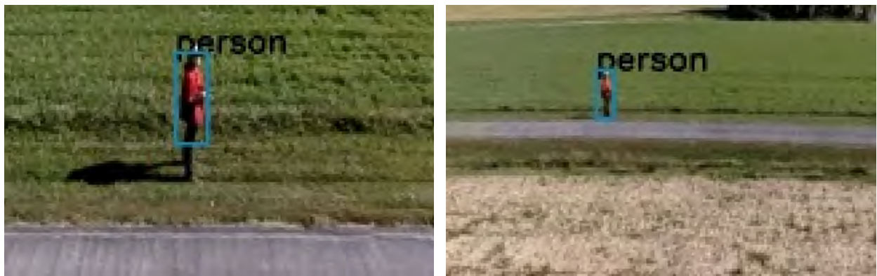
(a) The bounding box only encloses a portion of the body when the object is large. (b) The bounding box encloses the entire body when the object is small.
