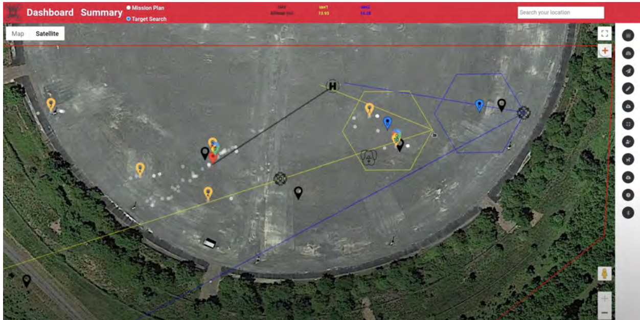
Fig. 12 Modified flight paths executed by the two UAS for revisiting the objects of interest.
