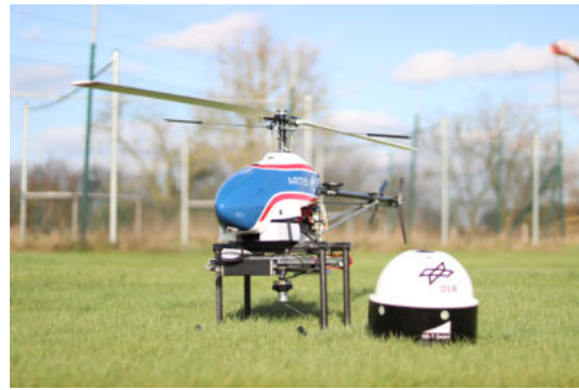
(b) DLR meARTIS demonstrator on the left, intelligent winch prototype on the right.
