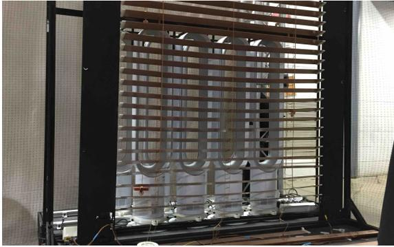
(a) Gust generation system consists of a set of eight Dyson fans behind remotely operated blinds
