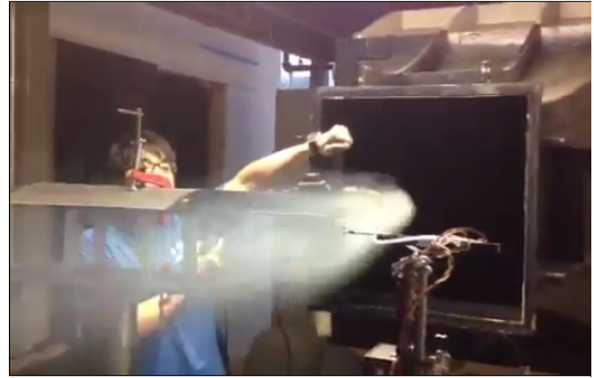
Figure 8. Introducing smoke into the wind tunnel flow. The resultant spreading of the smoke indicates that there is some change in the flow across the airfoil.
