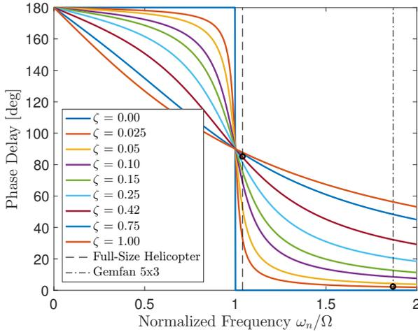
**FIGURE 3: BLADE-FLAPPING PHASE DELAY IN HOVER (ADAPTED FROM [17])**
