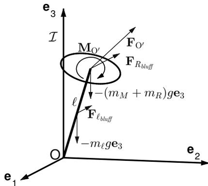
FIGURE 7: ROTOR-PENDULUM FREE-BODY DIAGRAM
