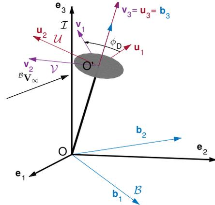
FIGURE 6: ROTOR-PENDULUM  $\mathcal{U}$  AND  $\mathcal{V}$  FRAMES
