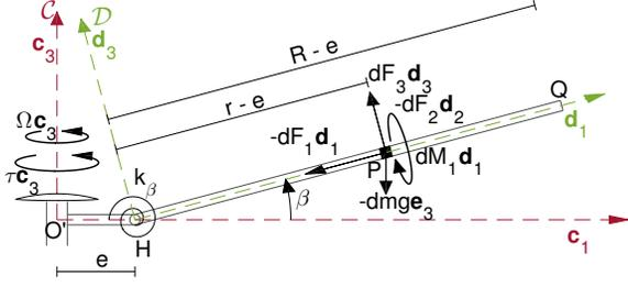
FIGURE 2: FREE-BODY DIAGRAM
