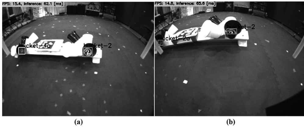
Fig. 13 Inspection framing comparison: filtered estimate (left) versus first AprilTag estimate (right).
