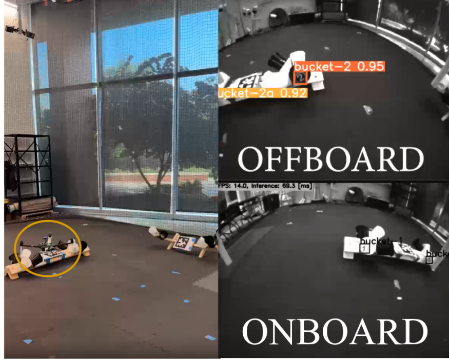
Fig. 8 Onboard vs. offboard inference delay. The UAV’s actual position (left) is compared to the object detection running on the ground station (offboard) and on the drone’s companion computer (onboard).
