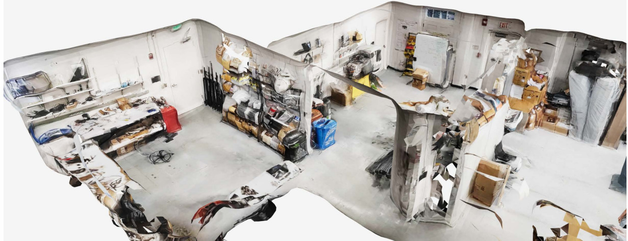
Fig. 23 Another view of the map showing the quality of textural details captured by the custom-developed low-cost multispectral mapping sensor system.
