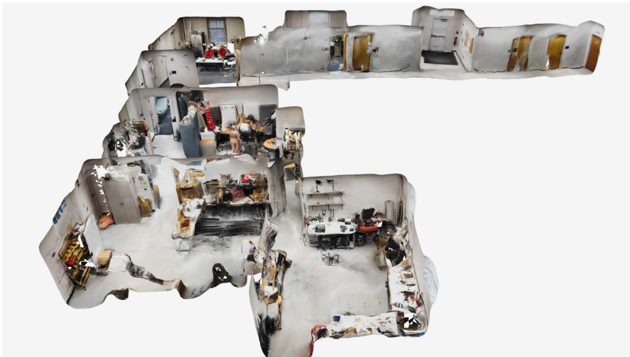
Fig. 22 Detailed post-processed map of a set of cluttered interconnected rooms and a narrow corridor of a building at UMD.
