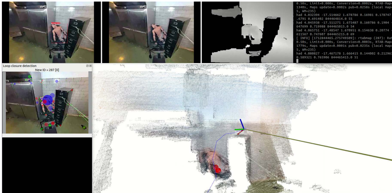
Fig. 18 Real-time detection and localization of a person manikin
