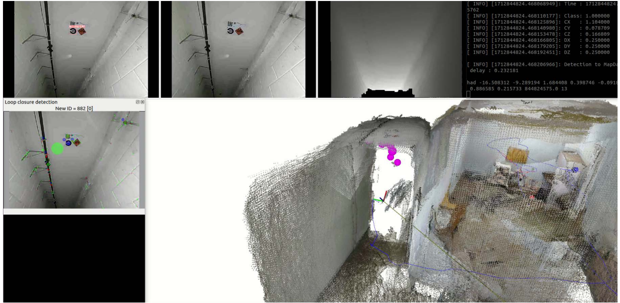
Fig. 19 Real-time detection and localization of a NIST ring target
