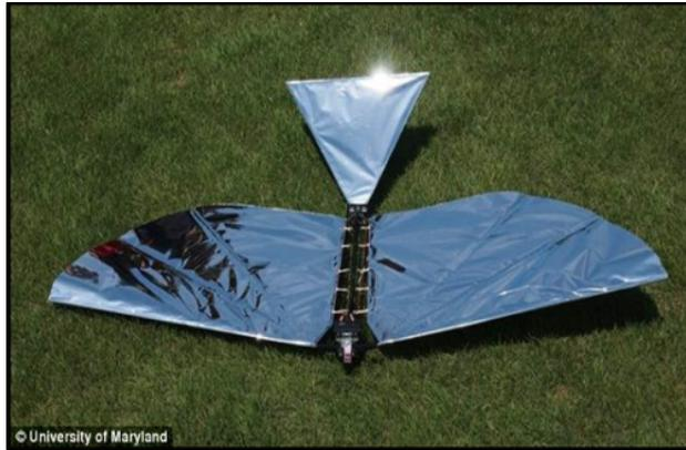
**Fig. 3** RoboRaven is a flapping wing UAV developed at the University of Maryland [25].
