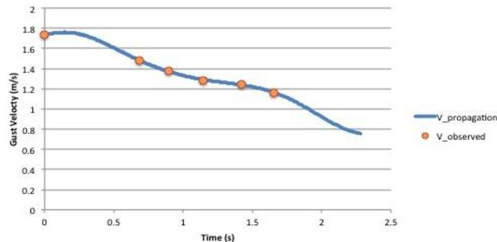
Figure 11. Gust velocity decay model
