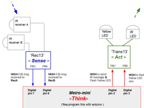
Figure 3: FIREfly system overview (from AUSS training manual)
