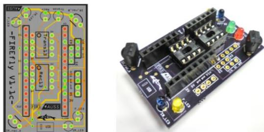
Figure 4: AUSS FIREfly version 1.1c
