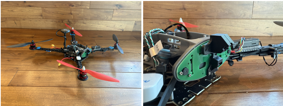
Figure 3.1: A-HAT-TRIC aerial platform with camera mount
