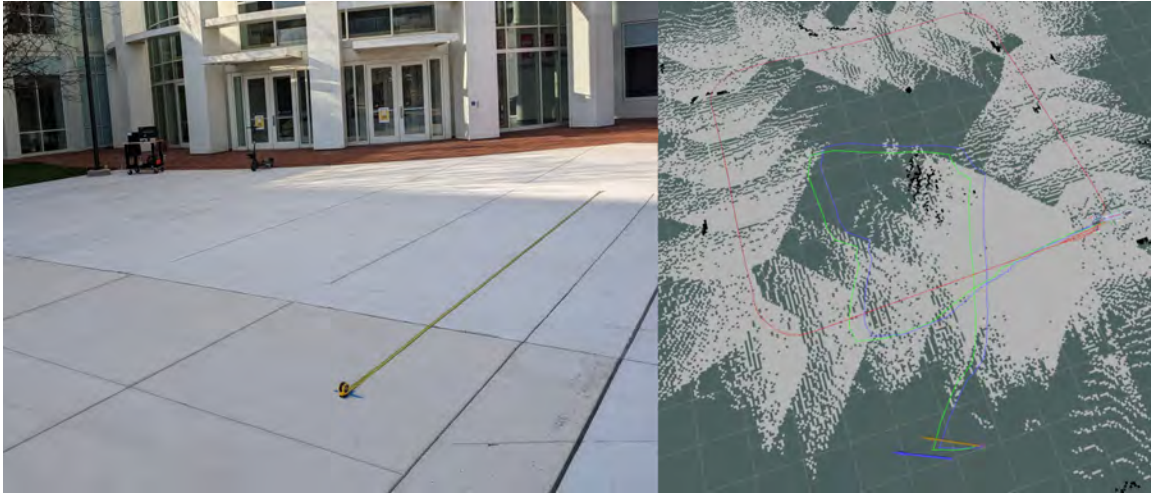
Figure 4.4: The scooter is made to follow an 8x8m square in Kim Plaza, a low feature environment. The figure on the right shows the output of our local EKF (Wheels and IMU) in red, and the ZED's odom and pose outputs in blue and yellow/green. The local EKF output follows the square well, but the ZED's tracking suffers.
