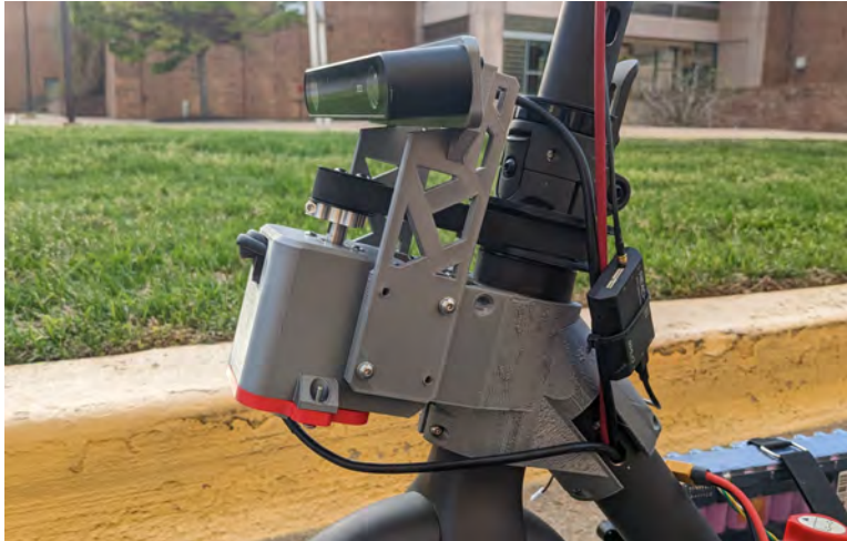
Figure 3.6: The new motor steering mechanism on Richard Parker is a big improvement over the previous, fixing any sagging or turning issues.
