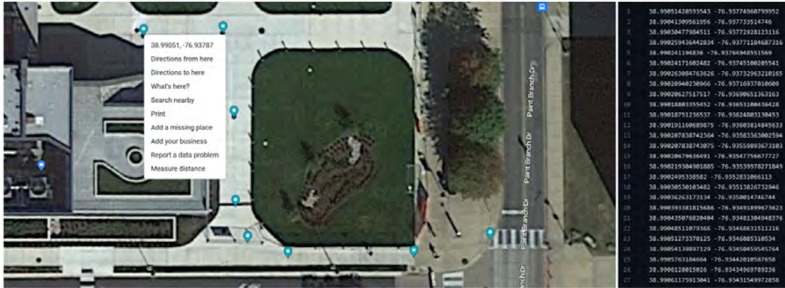
Figure 4.9: Screenshots showing the manual generation of waypoints from Google Maps into a text file which is later read by the autonomy stack. I also save the waypoints as labels (blue pins) for reference.
