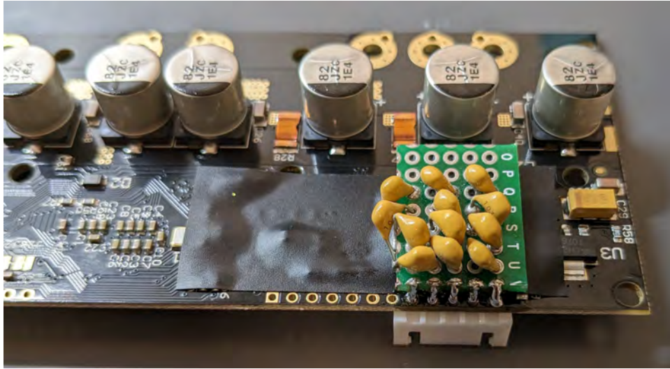
Figure 3.15: Noise decoupling capacitors were added to the hall effect encoder pins close to the ODrive.
