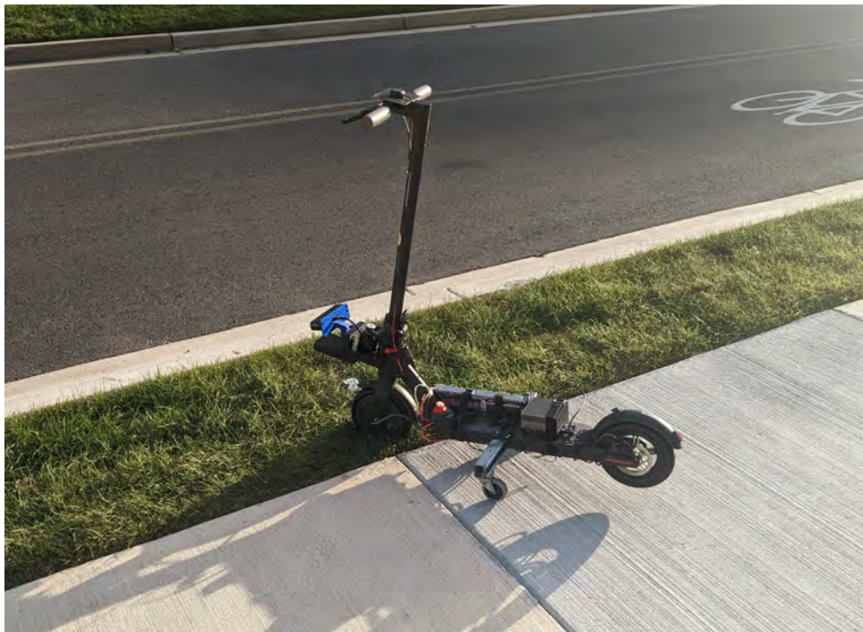
Figure 5.14: The scooter drives into grass and get stuck during an autonomous mission.
