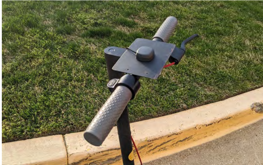
Figure 3.11: A picture showing the placement of GPS antenna with the metal ground plane added at the bottom to reduce multipath.
