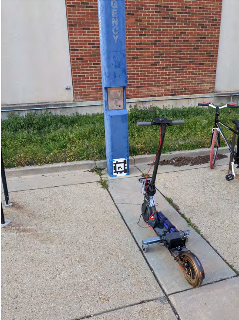
Figure 5.2: The scooter is started facing an AprilTag placed at a location which is identifiable on Google Maps, and therefore at a known global pose.
