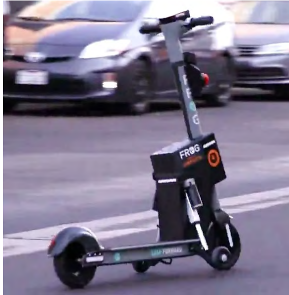
Figure 1.4: A teleoperated scooter by JUMPWatts for remote fleet management. Also seen is the dockable red charging port in the front.
