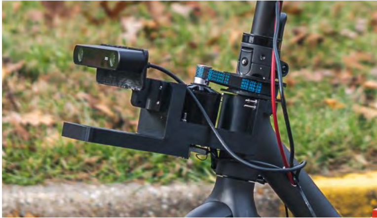
Figure 3.5: The old motor steering mechanism on Richard Parker
