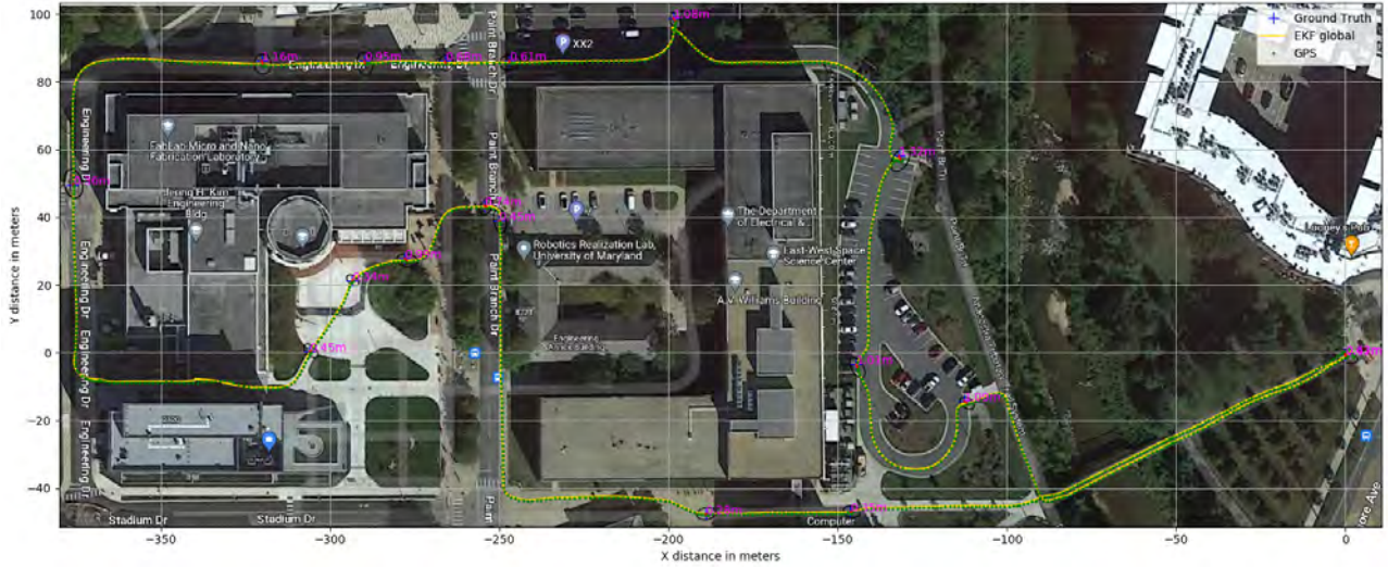
Figure 5.6: [Looneys Loop] The plot shows results of pushing the scooter manually along a known path to evaluate EKF performance - Path length 1150 meters. Black ellipses represent the covariance ellipse of the global EKF at the ground truth point, and the text in magenta is the distance error.
