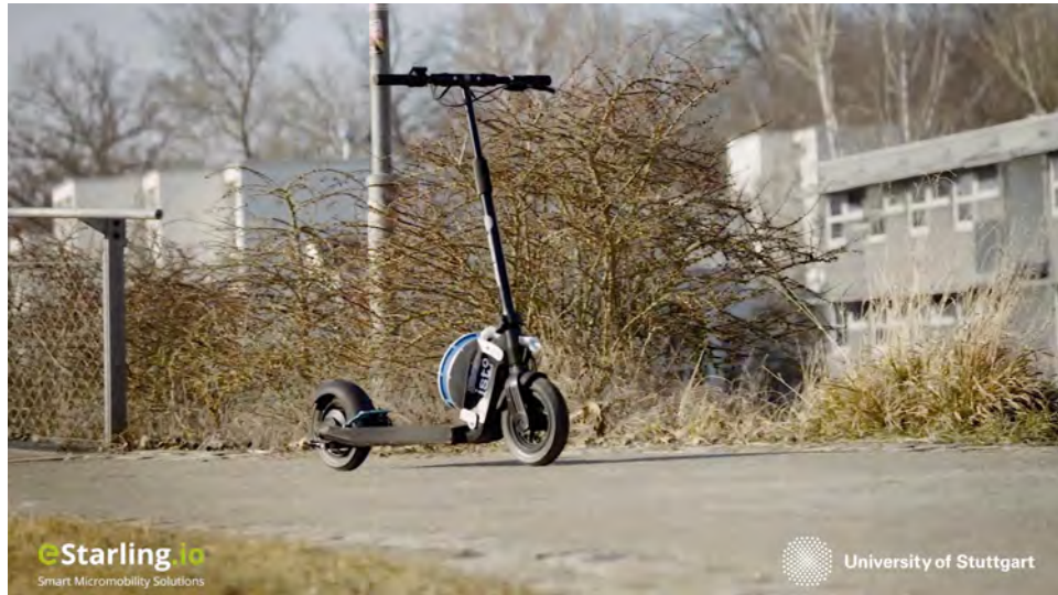
Figure 1.2: Researchers at the University of Stuttgart have presented their scooter self-stabilizing using a reaction wheel[4].
