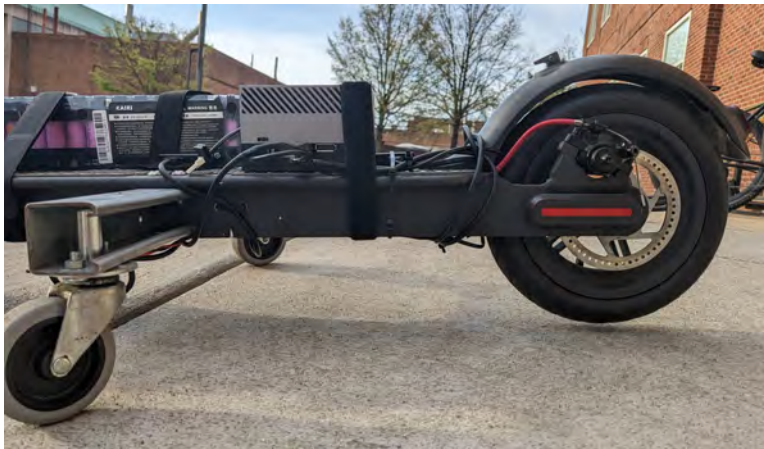
Figure 3.7: The rear wheels on Richard lift off the ground over certain uneven surfaces because of the stiff support wheels on either side.
