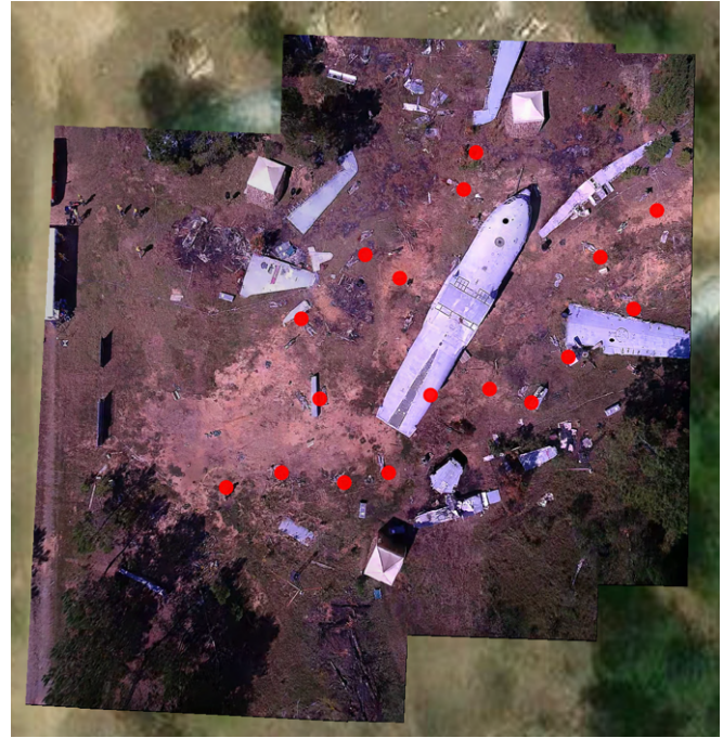
Fig. 8. Mission mosaic overlay for the DTC plane crash scenario with geolocated casualty markers overlaid.
