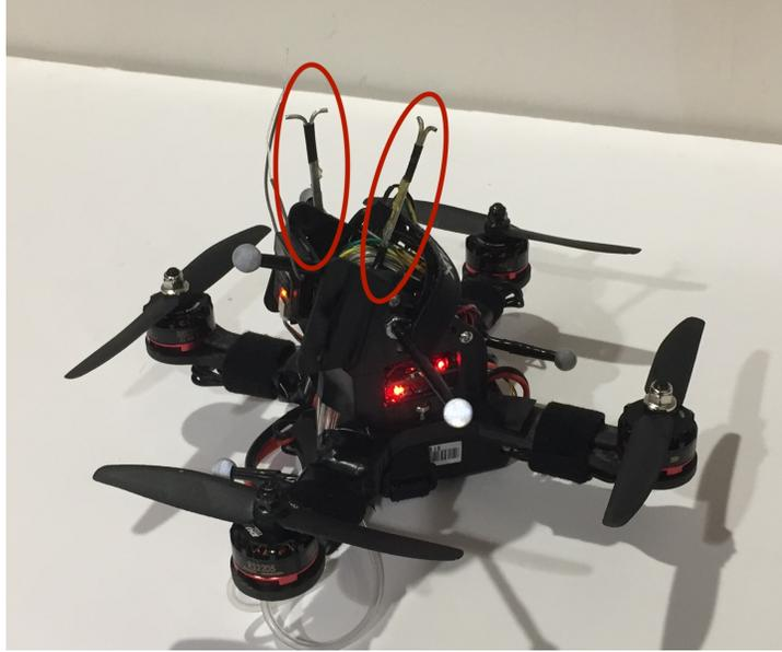
Figure 2.3: Experimental quadrotor vehicle with flow probes circled in red
