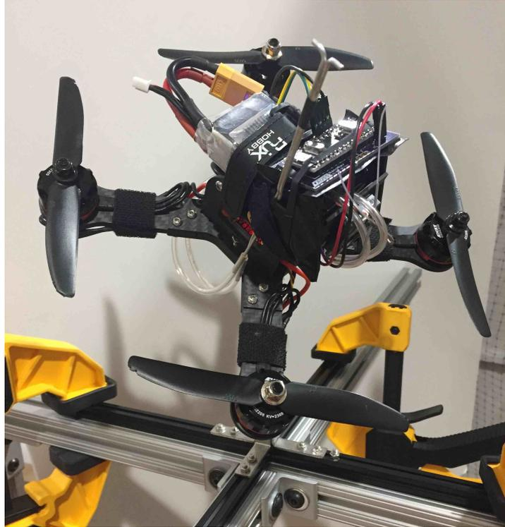
Figure 6.1: Quadrotor experimental attitude test stand
