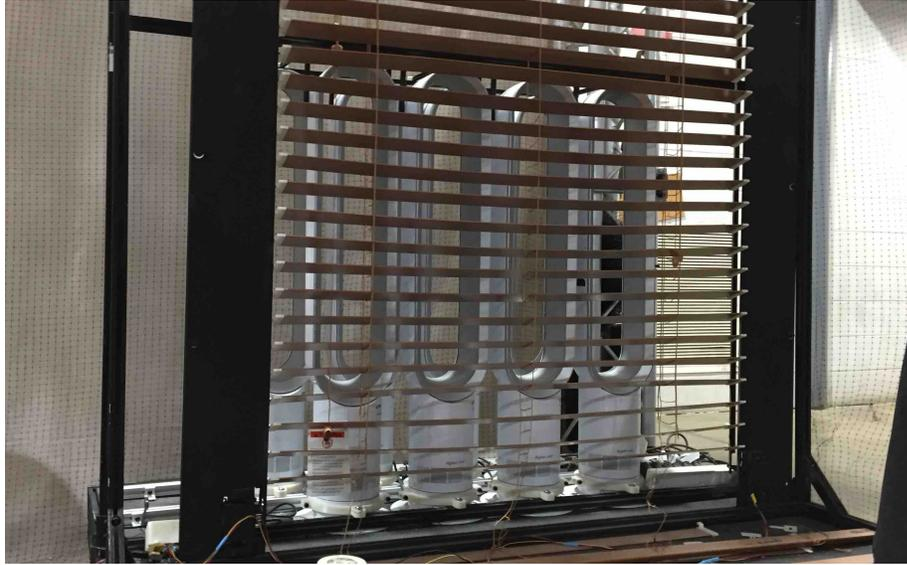
Figure 2.6: Gust generation system consists of a set of eight Dyson fans behind remotely operated blinds
