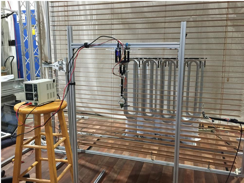
Figure 3.10: Test stand with gust generation system
