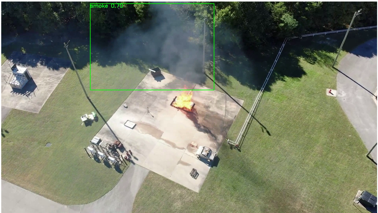
(a) An annotated Zenmuse H20 image with detected smoke.
