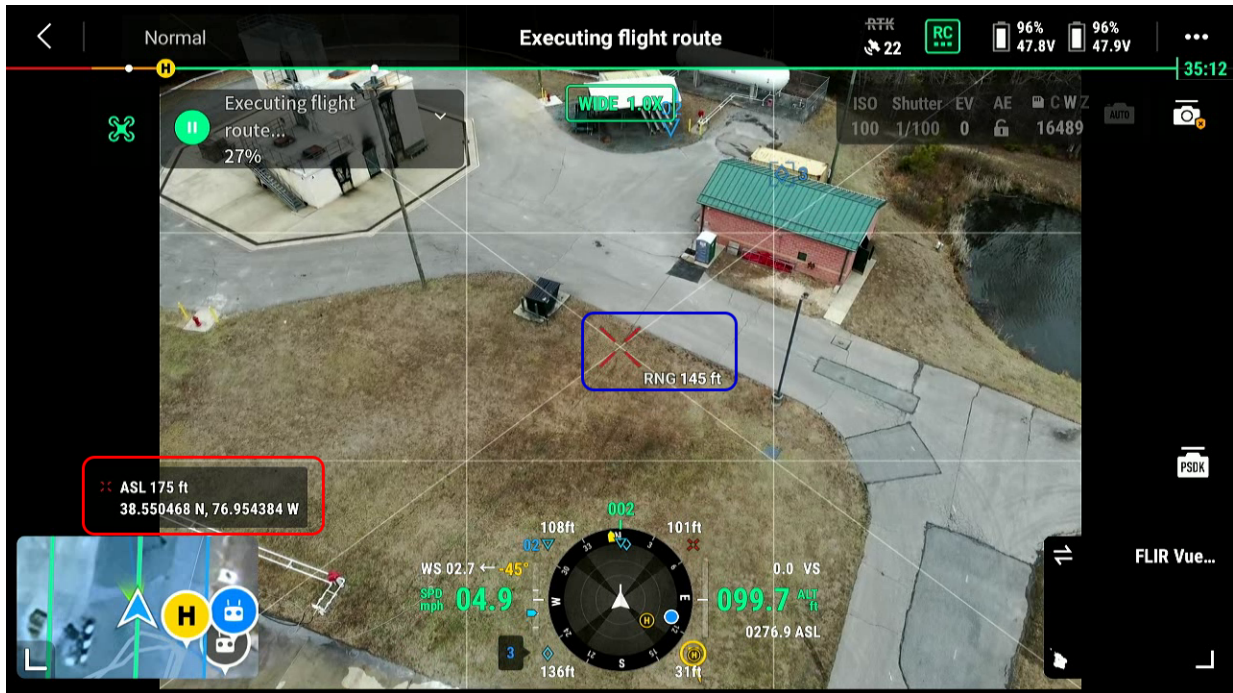
Figure 3.11: M300 RGB Camera stream with laser rangefinder position estimates circled in red and the rangefinder “target” and reported range circled in blue. Imagery taken at MFRI La Plata, February 5, 2025.
