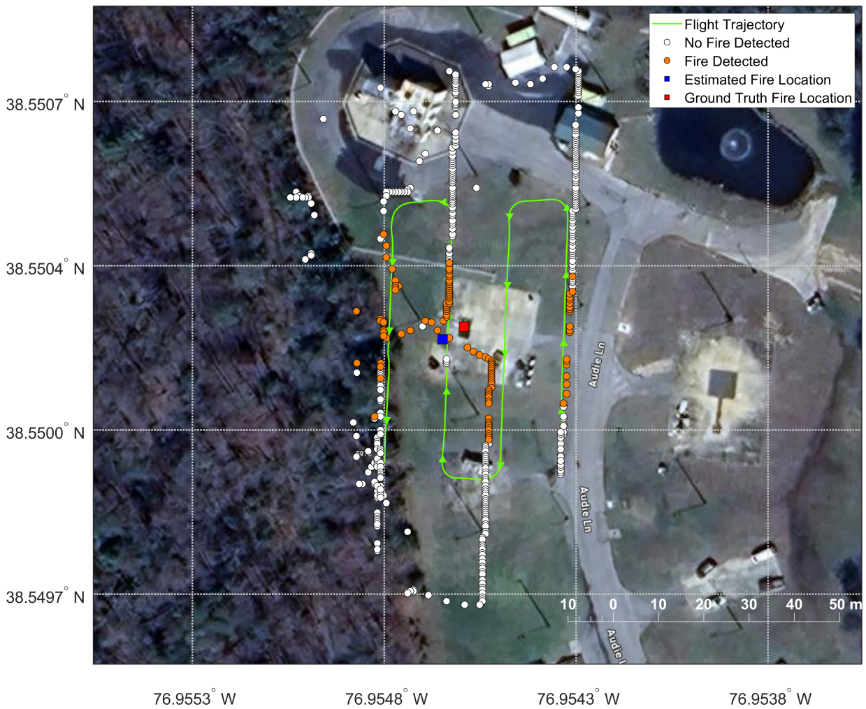
Figure 4.5: Detections and Flight Trajectory from broad area survey of a singular pool fire at 100 ft. AGL, thermal camera calibrated via fire. Test Date: February 5, 2025.
