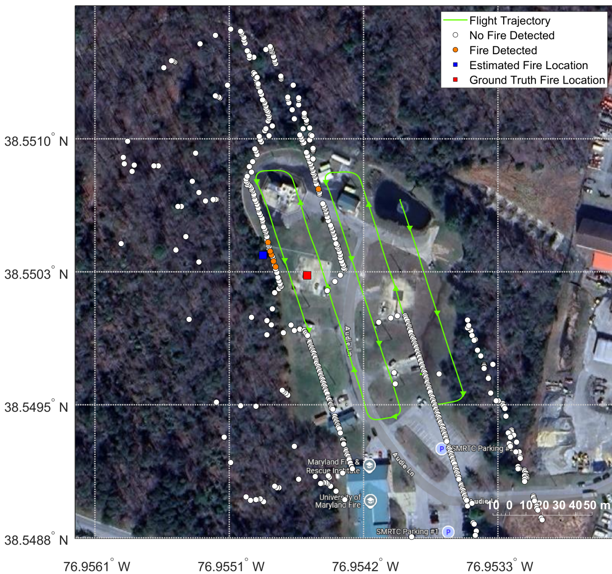
Figure 4.11: Detections and Flight Trajectory from broad area survey of a pool fire at 300 ft. AGL, UAV Velocity = 10 MPH. Test Date: March 26, 2025.
