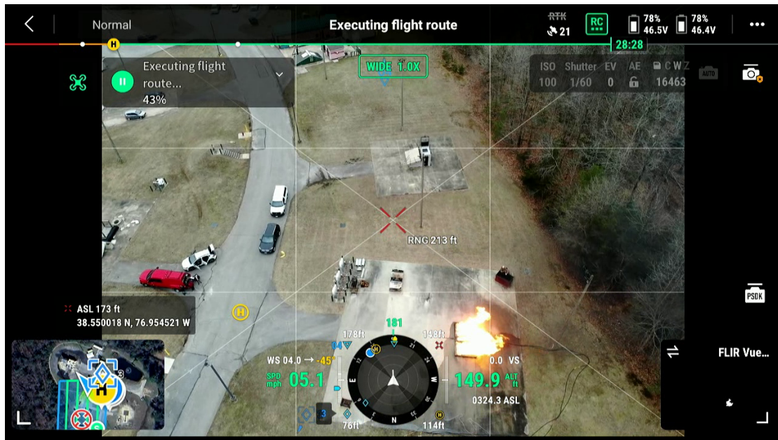
(a) A sample image frame of the RGB video live-stream with telemetry overlay.
