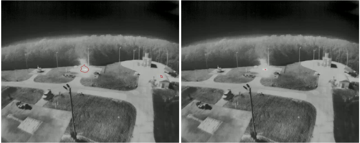
(c) Image from 3.2a annotated with a bit threshold of 180. (d) Image from 3.2a annotated with a bit threshold of 210.
