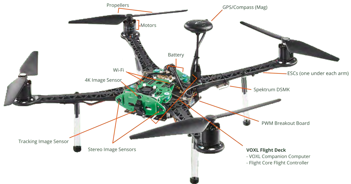
Figure 2.5: m500 drone setup with key hardware components labeled
