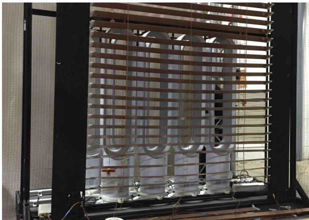
Fig. 3. Gust generation system consists of a set of eight Dyson fans behind remotely operated blinds
