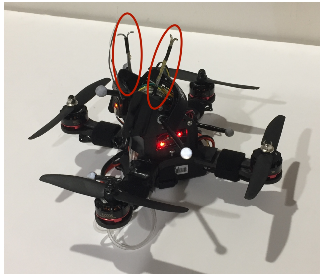
Fig. 1. Quadrotor used for experimental testing with flow probes highlighted in red
