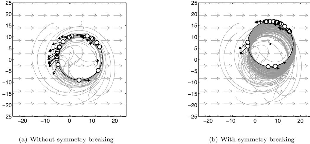
**Figure 2.** Stabilization of circular motion with  $N = 20$  and flow speed,  $\beta$ , equal to 75% of the particle speed relative to the flow. Without symmetry breaking, the particles converge to a circular formation with an arbitrary center. With symmetry breaking, the particles converge to a circular formation with center equal to the reference point  $c_0 = 6.7 + i6.8$ .
